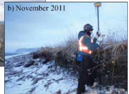
A team from the AK Dept. of Natural Resources takes repeat measurements for elevation profiles in Unalakleet.
