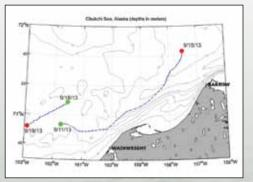
The acoustic glider traveled from Wainwright to Barrow in the Alaska Coastal Current where it was recovered at the beginning of Barrow's fall whaling season. The glider was redeployed northwest of Wainwright for an additional 2 days
