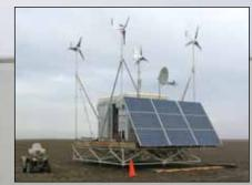
The Point Barrow shore station runs on wind and solar energy to power the radar in a remote setting.
