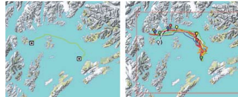
Drifter trajectories as measured from release time on July 25 at 02 GMT to recovery time on July 28 at 02 GMT (above, left) and as predicted by a cluster of ensemble ROMS forecasts (above, right).
