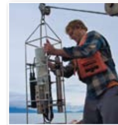
Experiment was fitted with a CTD sensor to measure the salinity and temperature of surface water as they traveled the Sound.
