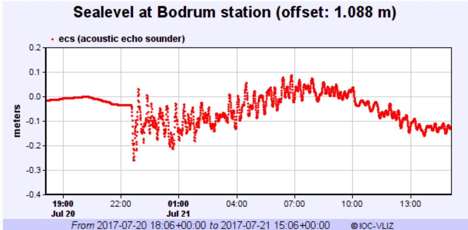
Datum referenced absolute measurements became non-referenced relative measurements after vertical displacement
