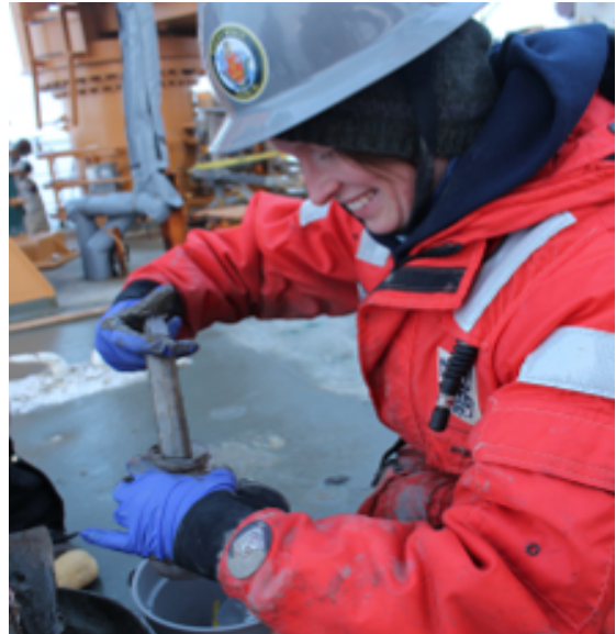
Collection of sediment plug from Van Veen grab used for abundance measurements of Alexandrium cysts
